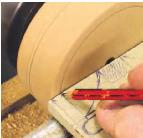
▲ Pic.10 Using the template, transfer all the relevant details onto the blank, both on the face and the side. If possible, use a hard pencil like a 4H; this will give you a crisper line
